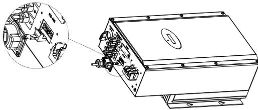
3. Lock the RS waterproof cover to the inverter casing and tighten the plastic nut clockwise, as shown below.
