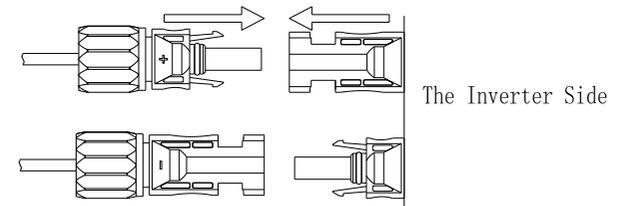
Notice that the connectors are in paired (male and female connectors). The connectors for PV arrays and inverters are H4 connectors;
