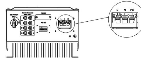
2.Unscrew the plastic nut of the AC waterproof cover counterclockwise, pull out the three rubber plugs, pass the three wires through the three holes on the waterproof cover, then crimp the OT terminal on the other end of the wire and screw the plastic nut. But don't have to screw it completely, as shown below.
