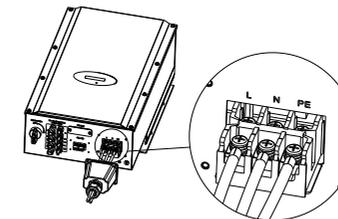
4.Lock the AC waterproof cover to the inverter casing and tighten the plastic nut clockwise, as shown below.
