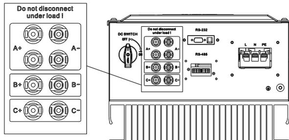
2. The PV connection wire is crimped to the corresponding PV+ /PV- metal terminals, and then plugging into the corresponding PV+ /PV- terminals, as shown below.
