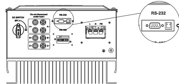
2. Plugging the monitoring module (WiFi/RF/GPRS Module) into the RS232 port of the inverter, and then screw the monitoring module to the inverter housing, as shown below.
