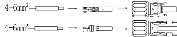
3. Plugging the connected wires PV terminals into the corresponding PV terminals on the inverter side, as shown below.
