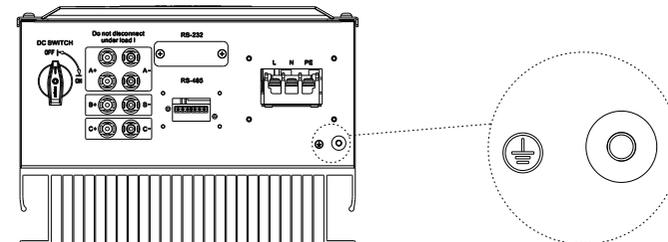
Crimp the grounding wire to the OT terminal, and then locking the grounding wire to the inverter housing by the cross combination screw, as shown below.
