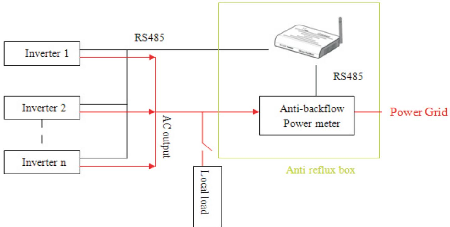
1) Each Webbox 5S monitoring reflux power ,After adjusting inverterrequires 15s to check again , When inverter output is adjusted, there's a time delay of 15s till the next anti-reflux monitoring(inverter adjusting time ).
