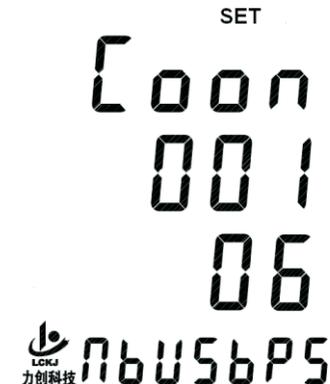
Figure 3.3 address and baud rate setting interface
